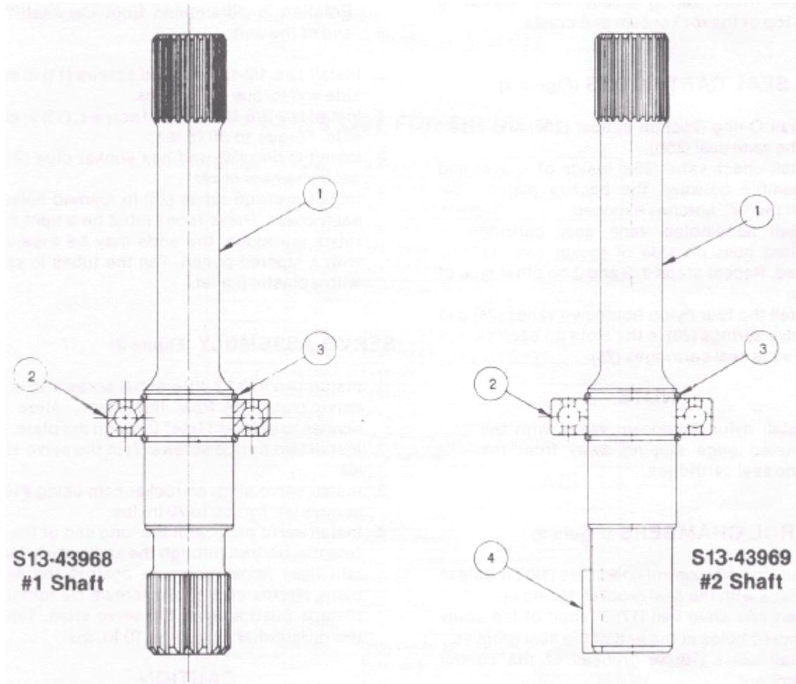
1. Pass one retaining ring (3) over the internal end of drive shaft (1) and install in the groove near the shaft seal surface. **DO NOT PASS THE RING OVER THE SEAL SURFACE.**
