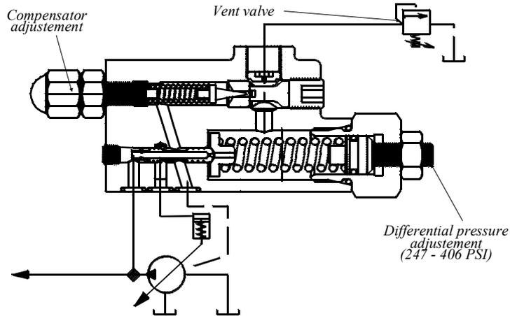
**L - LOAD SENSING COMPENSATOR**
