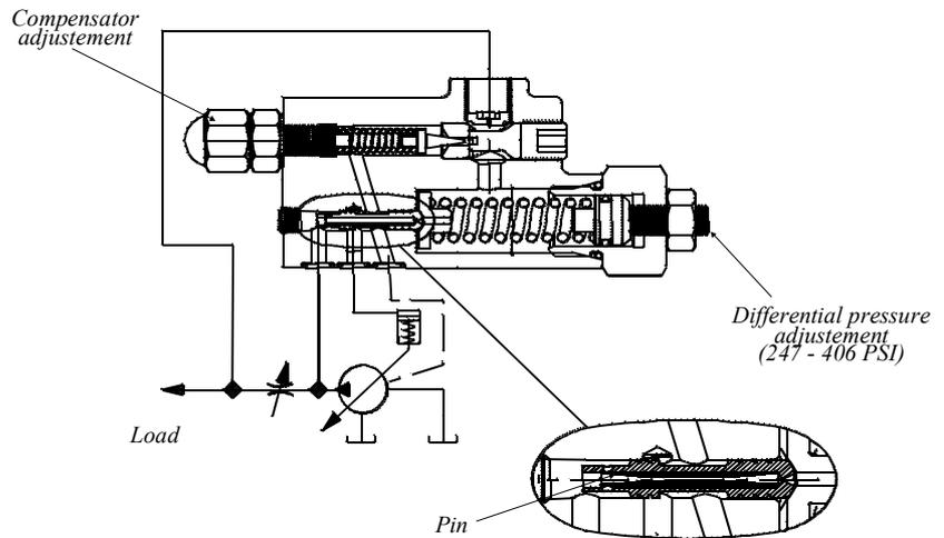
**X - VENTED COMPENSATOR BY ELECTRIC VALVE**
