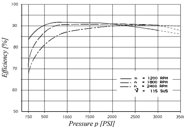
**INPUT HORSEPOWER - "P1" CARTRIDGE
